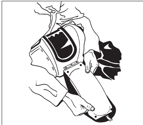
Fig. 3. Exchanging disposable window(s) Aspect
