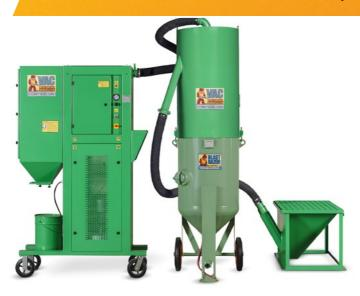
VAC-5 abrasive recovery system is an electrically operated vacuum suction system with an integrated high-performance cartridge filter with pulse-jet cleaning, an abrasive storage tank for automatic refilling of the blast pot (mounted directly on the Contracor Z-200 series blast pot), floor hopper, suction hoses.
