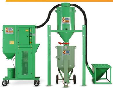
VAC-7H blast media recovery system is an electrically operated vacuum blast media recovery system, equipped with a 0.3 m³ free-standing storage silo and an extra powerful side channel blower. The VAC-7H Abrasive Recovery System can be universally used for recycling for further reuse or for a Big Bag filling station for disposal.
