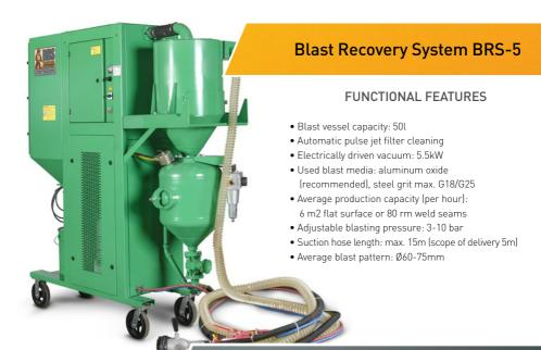
The BRS-5 Blast Recovery System is an electrically operated, pressure-feed closed-circuit blast machine, which can be used where open-air blasting is prohibited, or is not possible or practical. Blasting and simultaneous media recovery are initiated by pulling the DMH handle. Keeping the blast area clean allows the operator to blast without the need to encapsulate the area or wear respiratory protective equipment.
